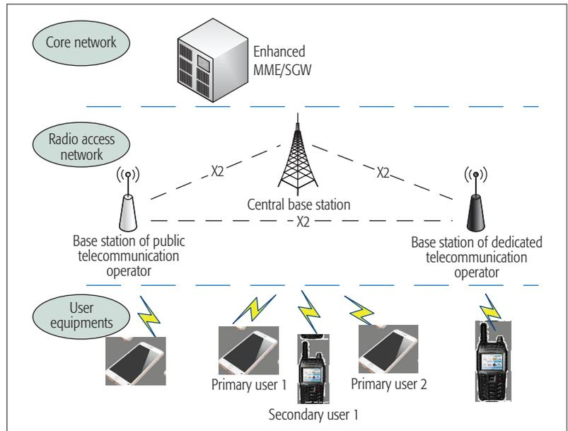
FIGURE 1. LTE-based 5G spectrum sharing system architecture.
