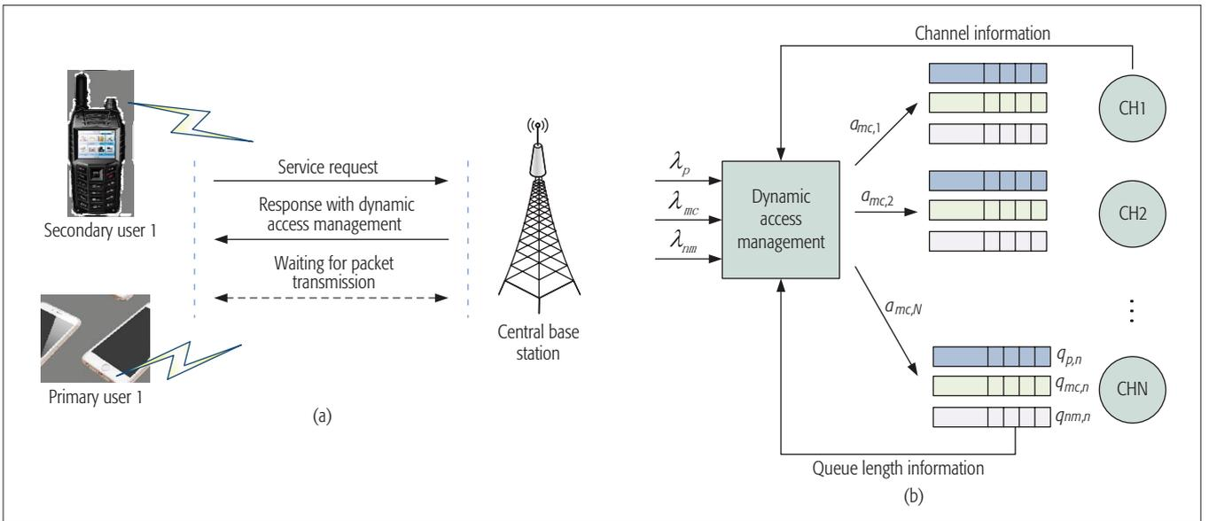
FIGURE 3. Dynamic channel access strategy in leasing spectrum: a) channel access procedure; b) queuing model for the leased spectrum.
