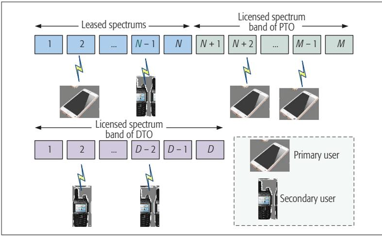
FIGURE 2. Spectrum allocation of PTO and DTO.
