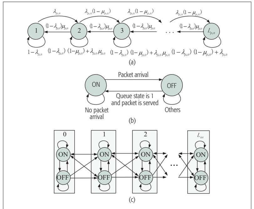
FIGURE 4. Queuing model for a PU and the NMS of an SU in leasing spectrum: a) queue state transition model for PU queues; b) channel service state transition model for PU; c) queue state transition model for MCS of SU queues.
