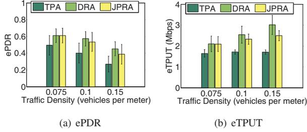
Fig. 3: Illustration of performance degradations due to negligence of the power-rate coupling.
