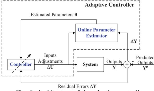
Fig. 6: Architecture of the adaptive controller.
