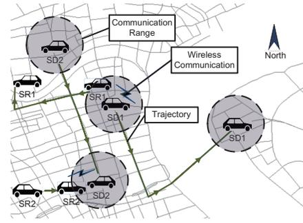
**Figure 1: An illustration of the distributed directory-based architecture in VANETs. When SRs meet SDs, they will send the query for a certain service. Then the SDs can reply the query by the service owner's id. If there are no SDs in the vicinity, SR will wait for some time delay until it encounters the first SD and gets its request answered.**
