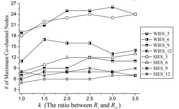
Fig. 4 Comparison of maximum co-channel nodes (i.e. the maximum interference level of SIES)
