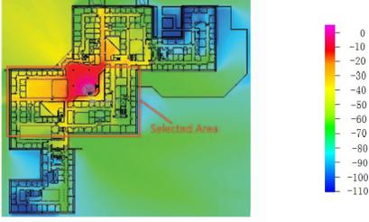
Fig. 3. RSS map for simulations measured in dBm.
