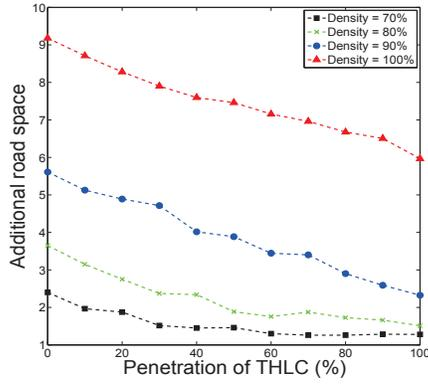
Fig. 13.  $\phi$ : Additional road space when  $p$  varies with  $Density$  fixed ( $q = 70\%$ ).
