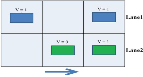
Fig. 1. Configurations in the NaSch model. (The number at the top denotes the velocity).
