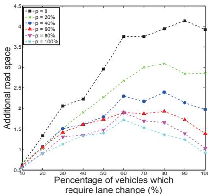
Fig. 15.  $\phi$ : Additional road space when  $q$  varies with  $p$  fixed ( $Density = 80\%$ ).
