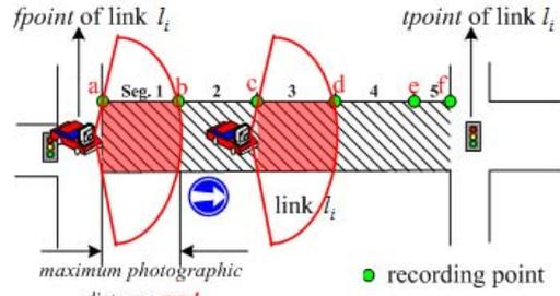
Figure 1. The illustration of maximum photographic distance
