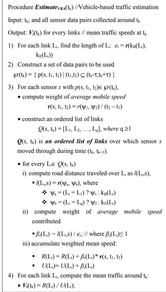
Figure 2. Vehicle-based algorithm for traffic estimation
