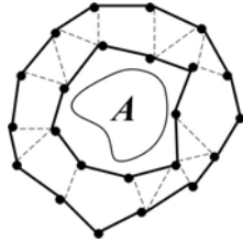
Fig. 2. Coverage graph of strong k -barrier coverage surrounding region A , where k = 2 .
