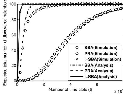
Fig. 7. Validation of analysis ( $N = 100$  and  $\theta = 0.1\pi$ ).
