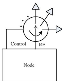
Fig. 1. Node architecture with sectored-antennas.
