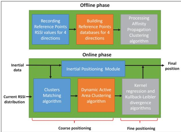
Fig. 4. System Block Diagram
