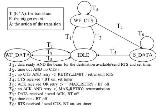
Fig. 3. The Finite State Machine of BT-DMAC
