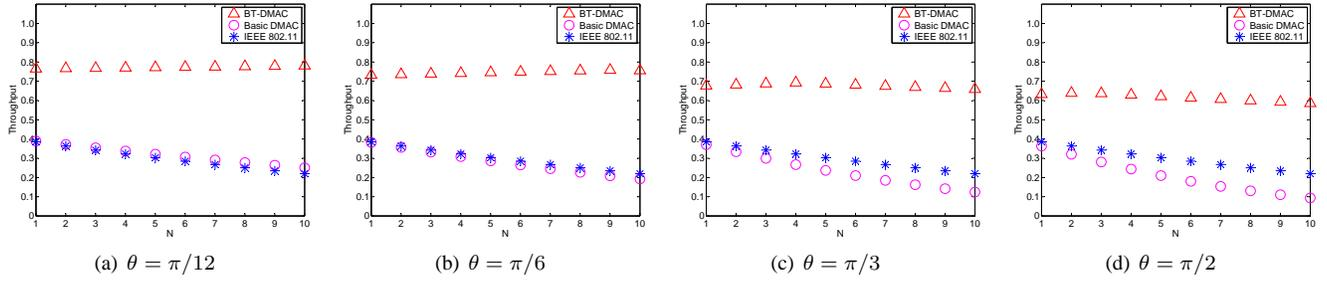
Fig. 6. Throughput comparison when  $\gamma = 1$  and  $p = 0.008$  ( $t_{rts} = t_{cts} = t_{ack} = 5\tau$ ,  $t_{data} = 100\tau$ )
