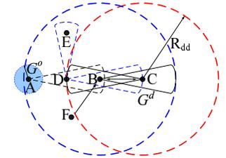
Fig. 5. BT-DMAC solves the hidden terminals and deafness problems
