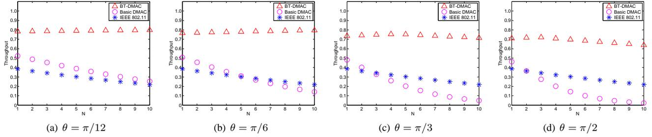
Fig. 7. Throughput comparison when  $\gamma = 2$  and  $p = 0.008$  ( $t_{rts} = t_{cts} = t_{ack} = 5\tau$ ,  $t_{data} = 100\tau$ )
