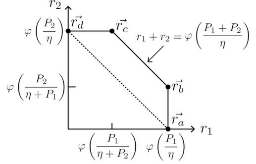
Fig. 1. Capacity region of a multi-access channel for a receiver node receiving data from two simultaneous transmitters. The region is upper bounded by solid lines. For a single user channel model, the capacity region is upper bounded by the dashed line.
