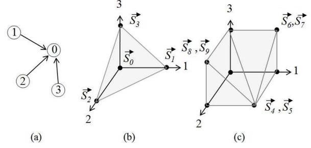
Fig. 3. (a) Network topology with three transmitter nodes and a receiver node. (b) Convex hull of characteristic vectors, assuming  $K = 1$ . (c) Convex hull of characteristic vectors, assuming  $K = 2$ .
