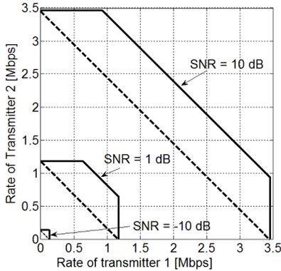
Fig. 7. Capacity regions of two transmitters located at a distance of 100 m of the receiver node.
